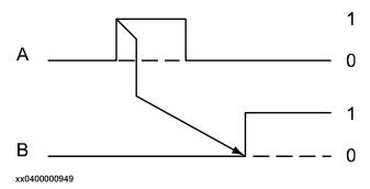
A: Load and Start (IN) B: Cycle On (OUT) 3.16.4.8 Motors Off
